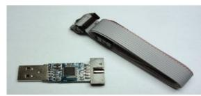
The AVR programmer will only be used once, to flash the gyro. Later a connection through the Servo plug will be used, to update the firmware and change the settings. There are plenty of AVR Programmers available. I can recommend the "USBASP". I got mine from Hong Kong through Ebay. Or you just buy it from HobbyKing, who just
