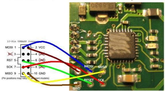
The soldered and ready for flashing gyro looked like this when I did it:
