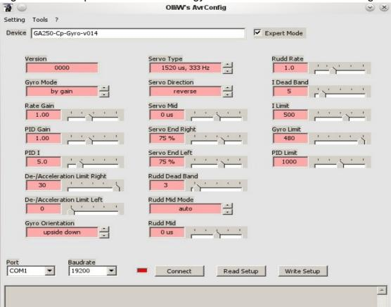
firmware folder. The gyro can be already installed in your helicopter. In the screenshot you can see AVRConfig with the default values. Plenty of parameters can be adjusted. For the beginning, you want to check:
