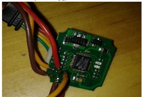
Soldering the wires on the tiny pads is not an easy task. Be careful when you are doing it. Use small wires, I used servo wire. Once you are done with the soldering, the hardware part is completed.
