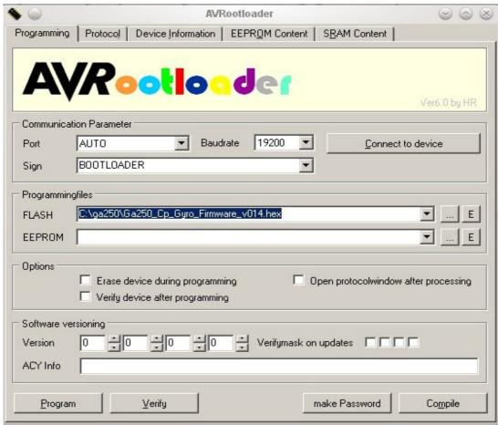
FT232) into the servo plug and press "Connect to device". Then connect the Lipo to your ESC and AVRootloader should show "connected".
